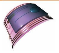
Human-interactive smart bandage: Touch sensors, temperature sensors, and a drug-delivery pump with a wireless coil are integrated on a flexible substrate and conformally covered surrounding human arm as a wearable device. The device can monitor real-time temperature and touch detections of human and drug curing.
